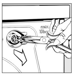
Use water pump pliers to withdraw the plastic filter by the bar (see illustration). Clean and put back.
